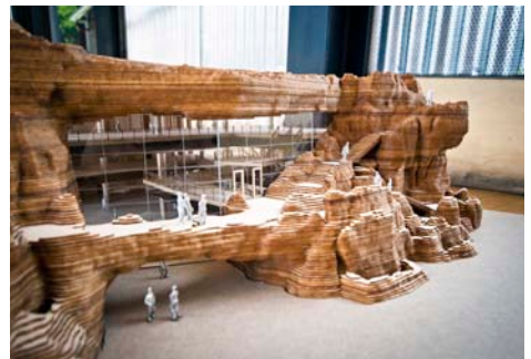
Laser Cut Model from 3D Scan
